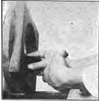
Fig. 234. Using Sandpaper on Frame.
